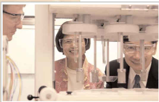
Bryan Katzenmeyer, analytic chemist, explains research capabilities of the newly dedicated Chao Center for Industrial Pharmacy & Contract Manufacturing to Lee-Hwa and Allen Chao. The center includes dissolution test equipment (shown) that can simulate human digestive conditions to fine tune pharmaceutical delivery. (Photo/Vincent Walter)
